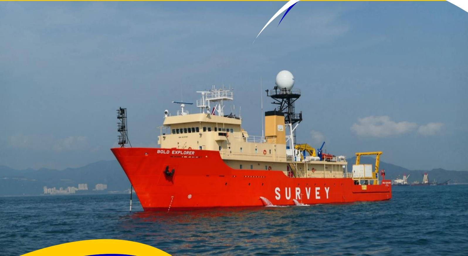
The Bold Explorer is a 68m multi-purpose geophysical and geotechnical survey vessel. This former Stalwart class vessel was fully refitted as a state of the art survey vessel in 2020, by EGS in Singapore.
