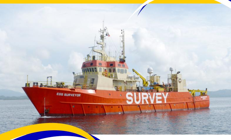
The EGS Surveyor is a 47m multi-purpose geophysical and shallow geotechnical survey vessel. This survey vessel was fully refitted as a state of the art survey vessel in 2010 & 2020 by EGS in Singapore.
