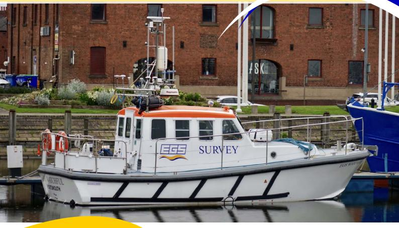
The EGS Watchful is a compact (overall length 10.1m, draft 1.1m) inshore survey vessel. The vessel operates under the MCA Workboat Code Cat 2 and is suitable for nearshore survey applications.
