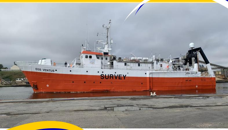
The EGS Ventus is a 50m multi-purpose geophysical and geotechnical survey vessel. The ice class vessel was fully refitted as a survey vessel in 2008, with further refurbishment in 2013.
