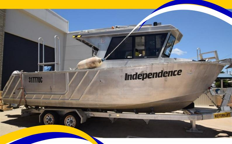
Independence is an eight meter inshore survey boat built in 2013. She has twin 200hp Honda four stroke engines and has a cruising speed up to 30 knots. Independence is equipped with an electric capstan and survey winches. Deployment is via a Maxilift
