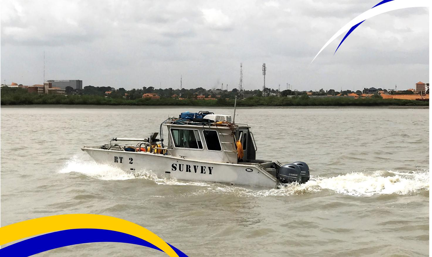
Survey launch RT2 is the daughter-craft of our research vessel Ridley Thomas. This versatile shallow draft vessel is fully equipped for near shore hydrographic, geophysical, oceanographic and environmental surveys. Amphibious survey boat capable of landing complete with moonpool.
